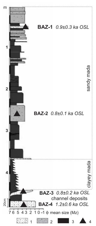
**Fig. 3**. Lithofacial section of the Vistula overbank deposits and OSL data of the samples taken from the research site on the Bazarowa Holm in Toruń.1 – sand, 2 – silty sand, 3 – silt or clay, 4 – points of taking samples for luminescence dating
